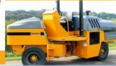
Pneumatic Static Compaction
